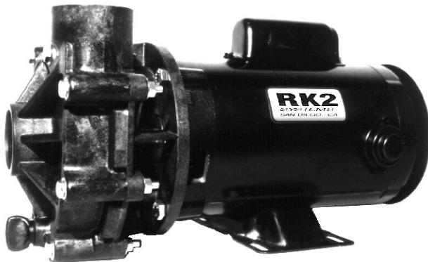
**RK2 Pumps are end suction centrifugal units that are close coupled to 56J motors. They feature excellent corrosion resistance with molded Noryl pump housings, 316 ss hardware, pump seals of Monel ceramic and buna, and motors with PVC encapsulated stainless steel motor shafts. Numerous electrical motor configurations are available.**
