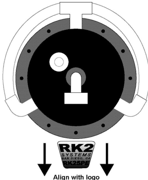
19. Place the top assembly on top of the second gasket, keeping the holes aligned and positioning it relative to the logo on the Reaction Chamber, as shown in Fig. 19.
