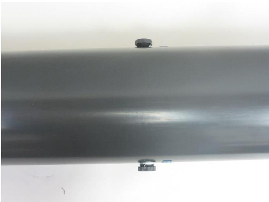
**Figure 3-20: Upper Auxiliary Port, and Lower Drain Port**
