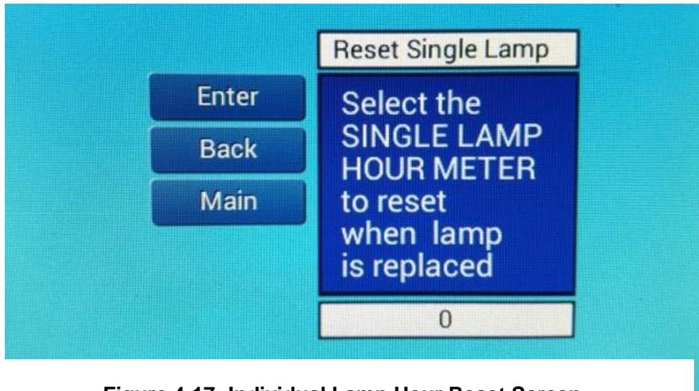
**Figure 4-17: Individual Lamp Hour Reset Screen**
