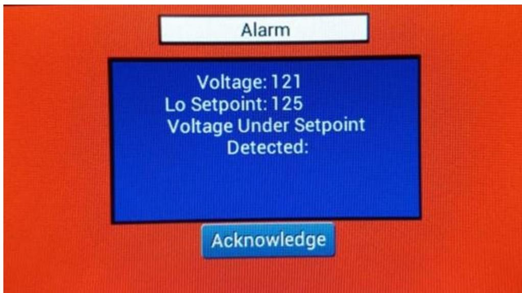
**Figure 4-30: Alarm Screen: Input Voltage Value Outside of Allowable Range**
