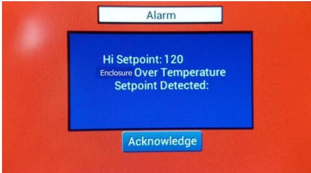
**Figure 4-31: Alarm Screen: PSE Enclosure Internal Temperature Limit Exceeded**
