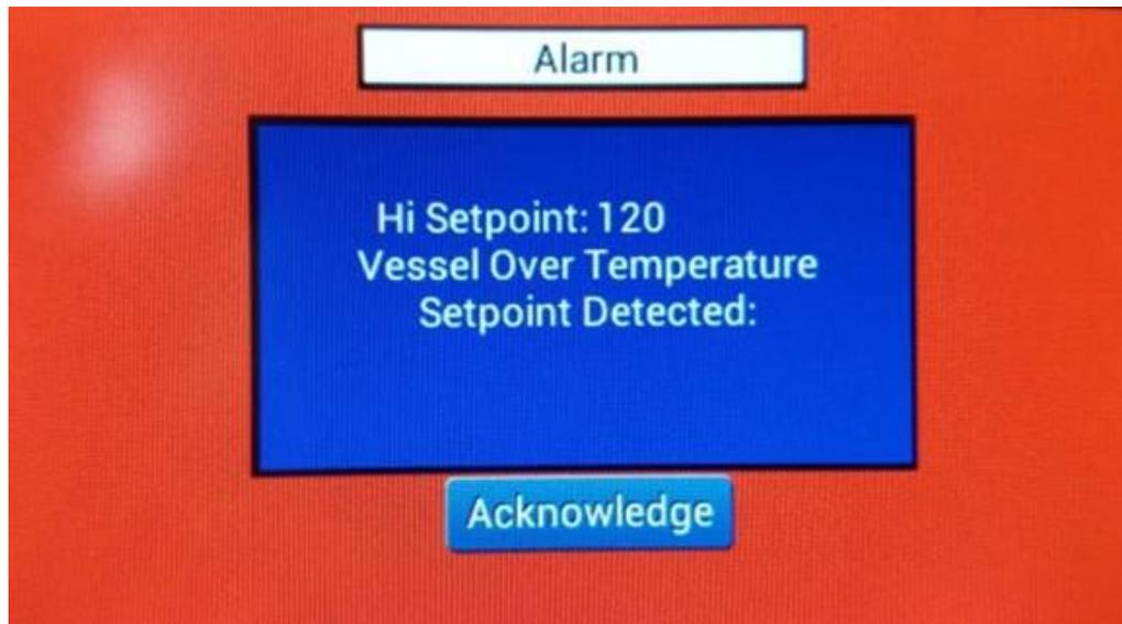
**Figure 4-32: Alarm Screen: Vessel Internal Temperature Limit Exceeded**
