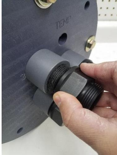
**Figure 3-4: Installing the Sleeve Assembly**
