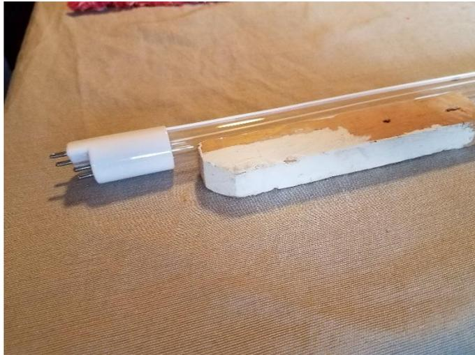
**Figure 3-19: Protective Paper, Anti-Rolling Device**
