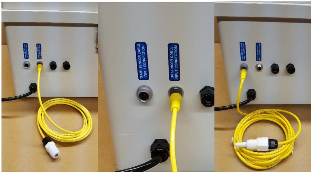
**Figure 2-10: Connecting the Sensor**
