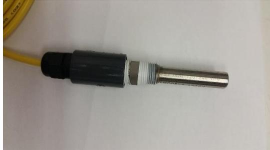
**Figure 2-7: Sealant tape on fittings**
