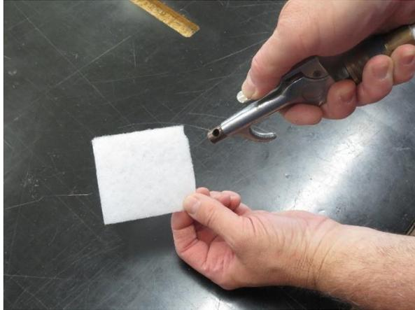
**Figure 3-22: Show blowing matt out with air PIC**
