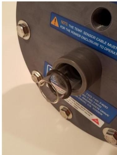
**Figure 3-1: Install Quartz Sleeves into the Reactor**
