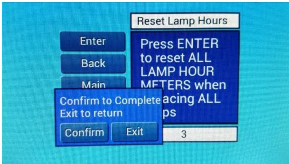
**Figure 4-16: Confirmation of ALL Lamp Hours Reset**
