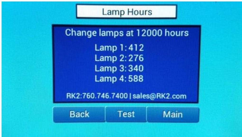
**Figure 4-28: Testing Individual Lamp Hours Display Screen**
