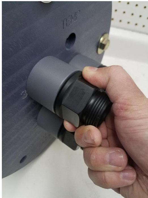
**Figure 3-6: Tightening the Sleeve Nut**
